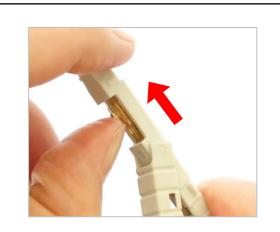
6. Slide V-groove holder and secure the inserted fiber.
