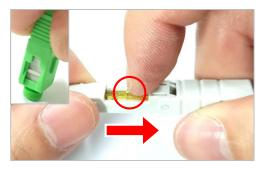
Push dust cap down and release the housing. Slide V-groove holder back and release the spliced fiber inside.
