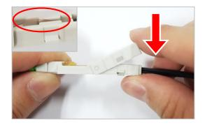
7. Please make sure that the micro-bending on the fiber remains and does not go over the connector body. If micro-bending goes over the connector, verify fiber cleaving length again. Close the boot clamp down. Verify the clicking sound to check the locking.
