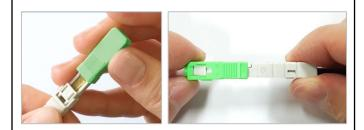
8. Affix connector housing to the connector body and complete the installation.
