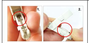
5. Insert the fiber into the hole as the box above. Stop inserting the fiber if micro-bending occurs on the fiber. Place and secure the cable(2x3mm) in the end grip of the connector body.
