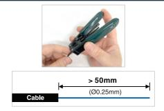
3A. Remove more than 50mm of 2x3mm flat cable jacket.
