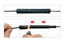
13. Place the heat shrink tube over the MSP. Apply heat evenly from the center to each end. Verify that no air remains inside the tube.
